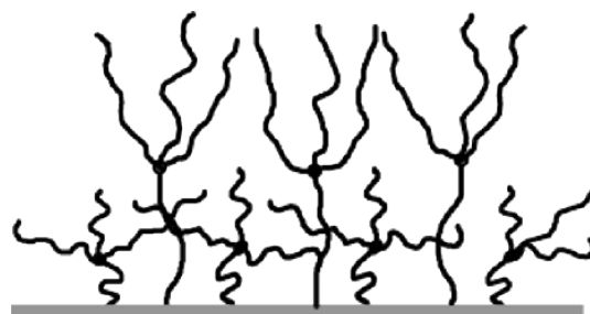
Figure 7. Schematic illustration of the occurrence of two populations of conformations of dendrons in a g = 1 dendritic brush.
